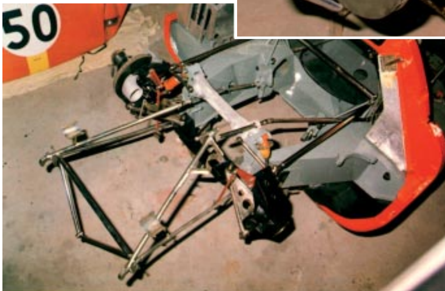
Engine bay and rear suspension of a Mark IIIb coupé.
